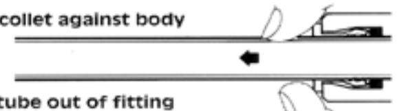
**Slide tube out of fitting**
