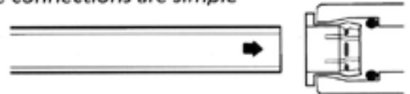
**Cut the tube square and push past the O-ring to the tube stop**
