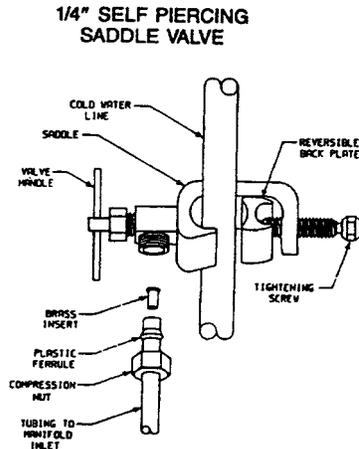
Do not over tighten the clamp. The clamp should be secure and resist a slight twisting force. Turn the saddle-tapping valve clockwise until the needle fully pierces the tubing and the valve seats. For maximum flow, back the handle out all the way. Adjust as required.
